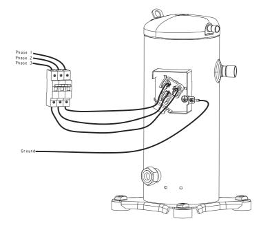
In the case of two-phase installations, it is mandatory to use a 2-pole circuit breaker, because in case of a short circuit both phases of power supply are protected. The system must be grounded.
