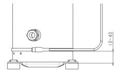
Crankcase heater is used to prevent refrigerant migration into the compressor shell during compressor off. It is suggested to be installed on all compressors for refrigeration application. It should be active at minimum 12 hours before the first compressor start and be active when compressor is off. This will prevent oil dilution and bearing stress on initial start up.
