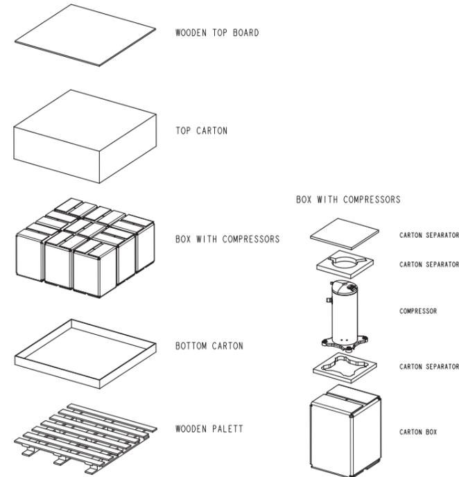
On compressor carton boxes are stuck labels with Bill of material code and Serial Number, including its bare code (Type 39).
