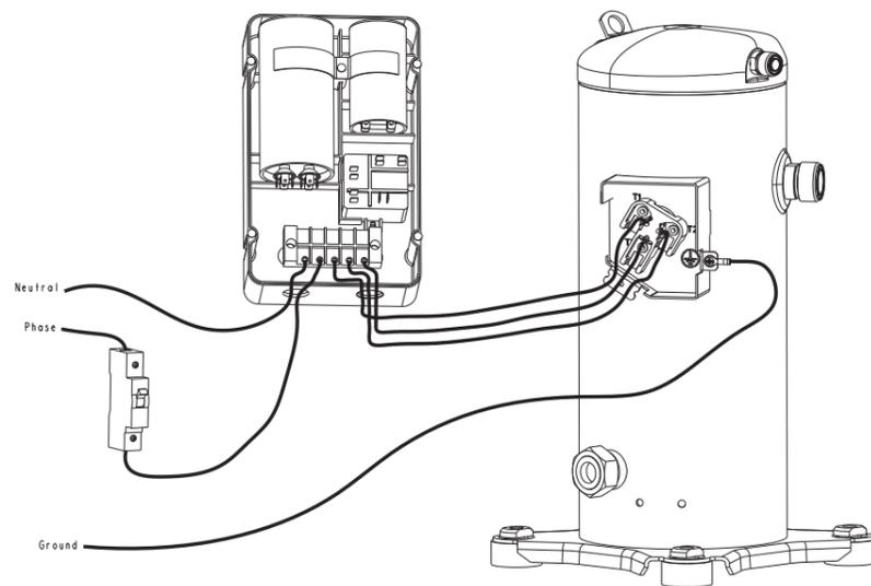
In single-phase installations with internal overload protector, the Phase wire must be protected by a circuit breaker and connected directly to common pin. The neutral wire must be connected to the relay starting device. The system must be grounded.
