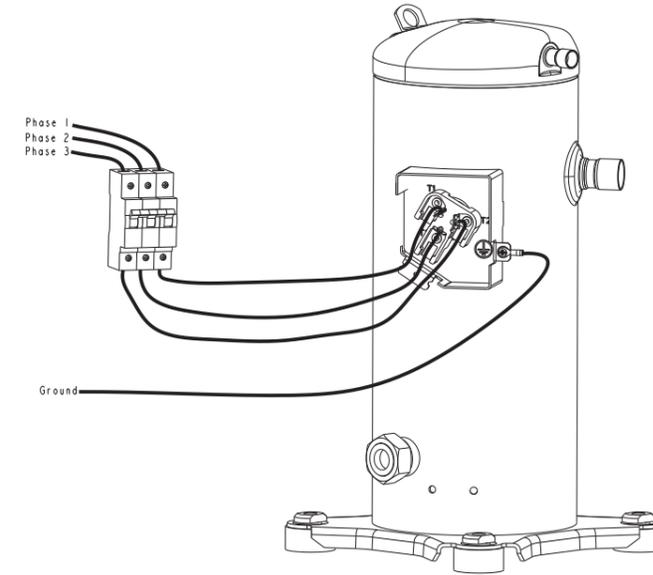
In the case of two-phase installations, it is mandatory to use a 2-pole circuit breaker, because in case of a short circuit both phases of power supply are protected. The system must be grounded.
