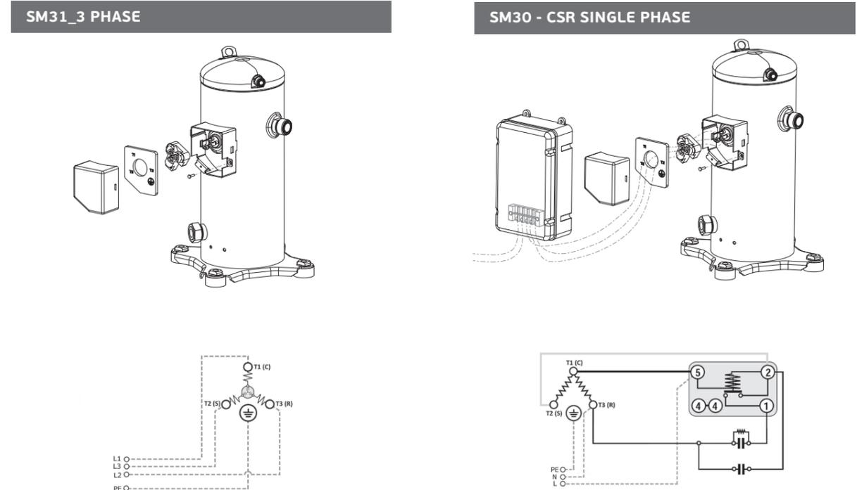
**Figure 10.3b Wiring diagrams keys**
