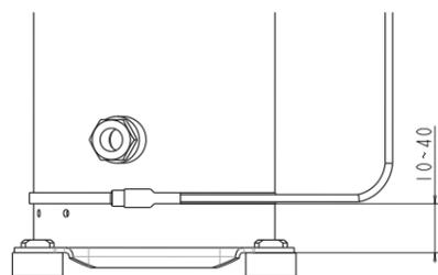
Crankcase heater is used to prevent refrigerant migration into the compressor shell during compressor off. It is suggested to be installed on all compressors for refrigeration application. It should be active at minimum 12 hours before the first compressor start and be active when compressor is off. This will prevent oil dilution and bearing stress on initial start up.
