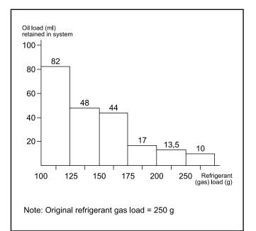
All previously listed causes can be directly or indirectly be related to the compressor low capacity symptom. Tests carried out by Embraco on compressors with a higher than normal oil circulation rate, did not reveal any impairment with the performance of the tested systems. Thus being, we suggest that all causes be investigated, step by step, emphasizing mainly those related to the refrigerant (gas) load.
