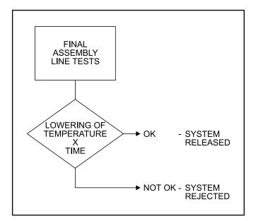
For a system to be rejected, it is necessary that the established parameter temperature is not reached within the determined time. Normally this system makes the compressor "suspect", as it is responsible for the product refrigeration and a premature judgment can result in it being condemned for "low capacity".
