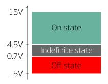
Figure 4.1: Signal levels for frequency control mode
