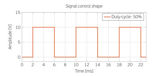
The compressor will follow frequency signal sent to the inverter according to the relation described on the following table and illustrated on the graph below.
