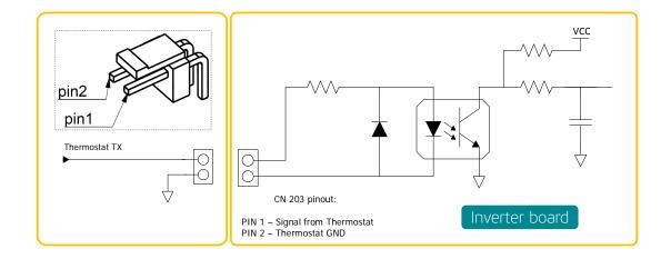
Figure 4.2: Electrical schematic of frequency communication
