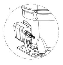
Figure 3.8: Step 6 - Screw the cord anchorage
