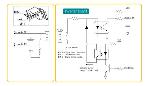
Figure 4.5: Electrical schematic of serial communication
