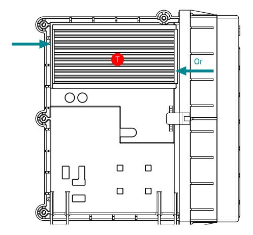
Figure 3.15: Inverter air flow direction
