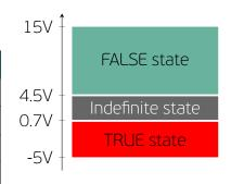
Figure 4.6: Signal levels for serial communication
