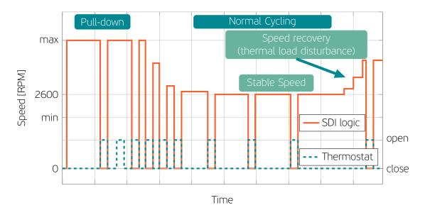
Figure 4.3: Compressor speed versus thermostat behavior Smart Drop-in
