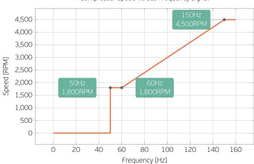
Compressor speed versus Frequency signal
