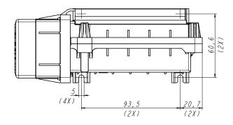
Figure 2.2: Stand alone dimensions (mm)
