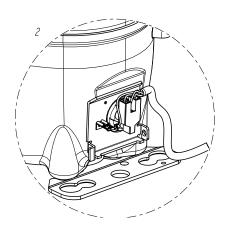
Figure 3.4: Step 2 - Connect the compressor motor cable
