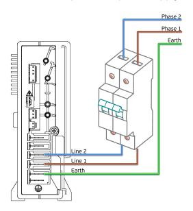
Figure 3.17: Phase-Phase connection
