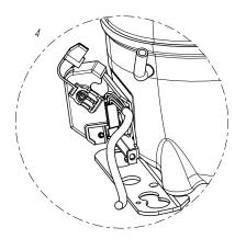
Figure 3.6: Step 4 - Assembly the fence cover
