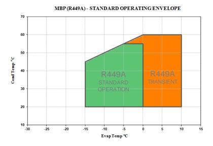
Figure 1. New limited operating envelope for R449A, return gas temperature 20°C, Evaporating range: -15 °C to 0°C for standard operation NEU/NT/NJ series
