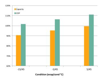
Figure 2. Calorimeter performance of R449A with baseline of R404A.
