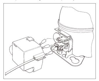
5 - Assemble the relay cover to the compressor.
