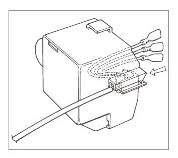
4 - Connect the phase, neutral and earthing wire terminals of the electric wire to the thermal protector, relay and compressor earthing terminal, respectively.
