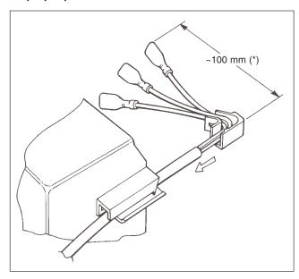
\* Proper place means that after assembling the cord relief to the electric wire, a gap will remain between the relay terminals and the cord relief.
