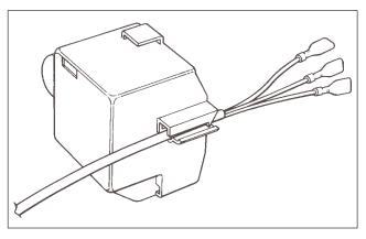
2 - Assemble the cord relief to the electric wire at the proper place\*.
