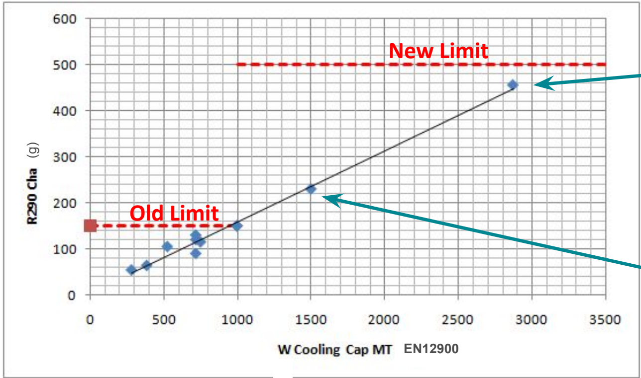
Typical R290 Charge In MBP Systems In Function Of Cooling Capacity
