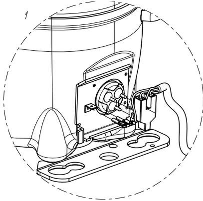
Figure 3.3: Step 1 - Connect the earth cable
