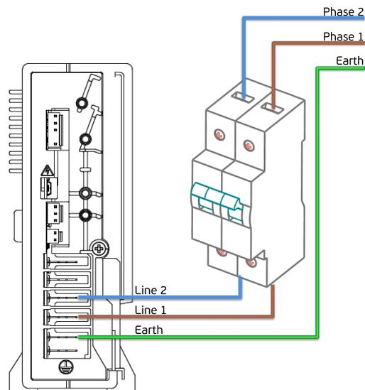
Figure 3.17: Phase-Phase connection
