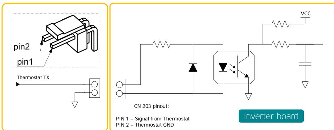
Figure 4.2: Electrical schematic of frequency communication
