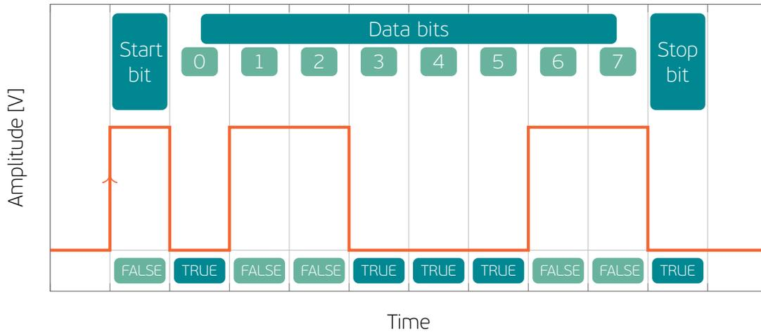
The identification byte (1st byte), is used for command synchronization. After inverter identifies a valid A5h, it starts to read the next 4 bytes. After reading, a response will be sent as indicated on "Receive commands structure" table. No response will be sent until the inverter recognizes a byte A5h. There is a time out of 2 seconds to receive the entire command after inverter identifies one A5h. After this time out, a new synchronization will start.
