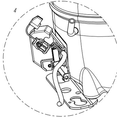
Figure 3.6: Step 4 - Assemble the fence cover
