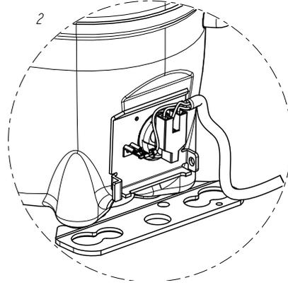
Figure 3.4: Step 2 - Connect the compressor motor cable
